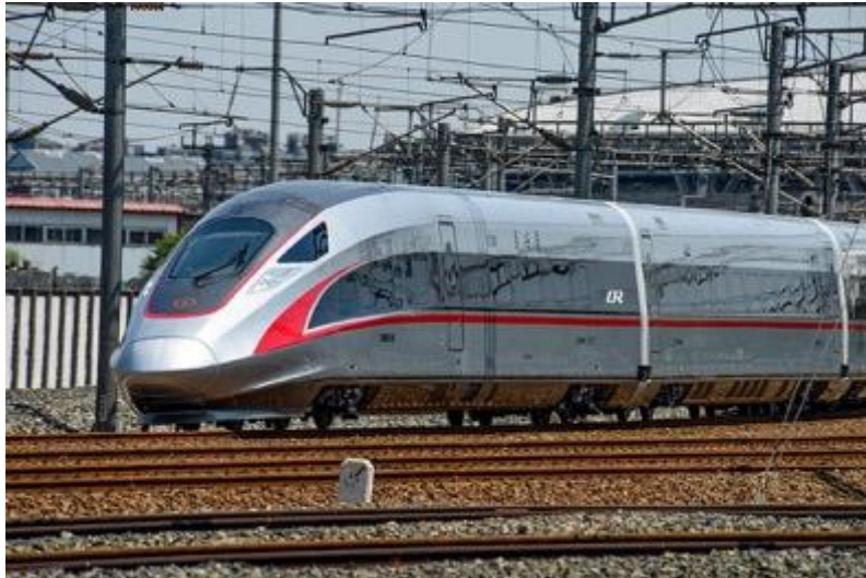
Figure 6.9. CRH CR400AF Fuxing Hao, electric multiple unit, used for the CRH fast delivery service; source: Wikimedia Commons, author: N509FZ, Creative Commons Attribution-Share Alike 4.0 International license
