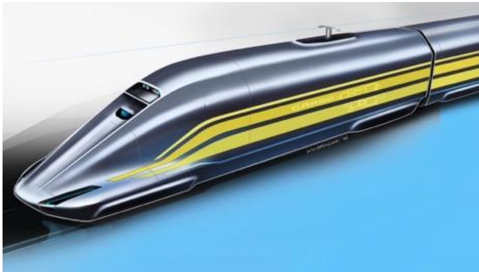
Figure 6.21. Next Generation Train Cargo (NGT CARGO), multiple unit with power car, source: DLR
