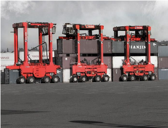
Figure 15: Straddle carriers used for stacking containers [Source: Kalmar industries]
