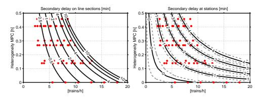
Figure 8: Contours of delay models using MPC as heterogeneity measure (black lines). Simulated values (red dots). Grey contours indicate the 95% prediction intervals.
