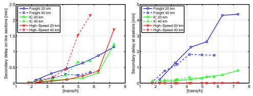
Figure 7: Results for timetable type 10, separated with respect to train type and infrastructure variant (20 km: solid / 40 km: dashed). Low primary delays.
