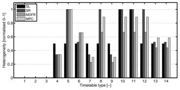
Figure 5: Normalised heterogeneity values for different timetable types. True range is: SL: 1-3 [-], SR: 1-1.77 [-], MDFR: 0-55 [min], MPC: 0-0.46 [h].
