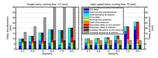
Figure 4: Results separated for individual train types in timetable type 5. Values for the bars ending outside the left figure are (left to right) 75, 82 and 62 minutes.
