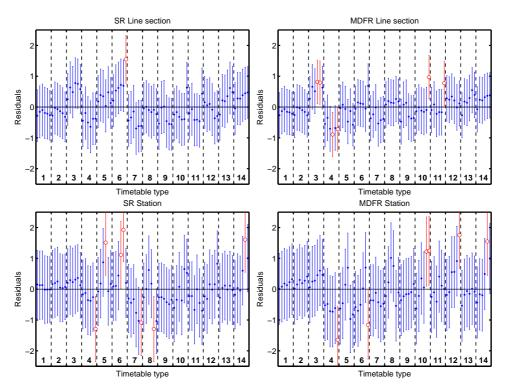
Figure 6: Residuals [min] for models using SR and MDFR. Line sections (top) and stations (bottom). High primary delay level. Negative residuals indicates that the model overstimates delays. Outliers are indicated in red color (95%). For each timtable type, traffic density increase in the rightward direction.
