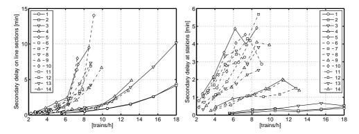
Figure 3: Secondary delays on line sections (left) and at stations (right).
