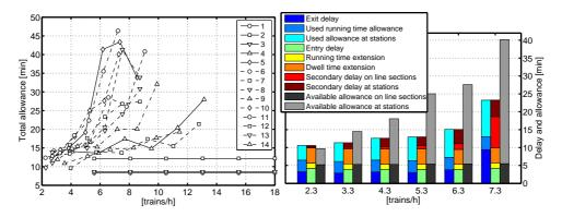
Figure 2: Left, total allowance for all timetable types as function of traffic density. Right, simulation results for timetable type 10 (high-speed, intercity, freight trains), mean values for all train types.
